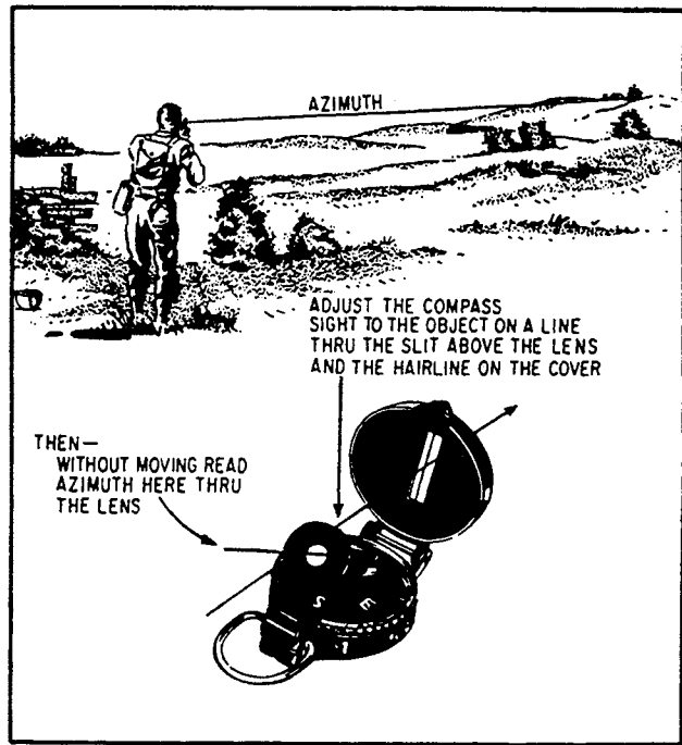
Figure 5-28.—A method of determining the azimuth of a visible object.
