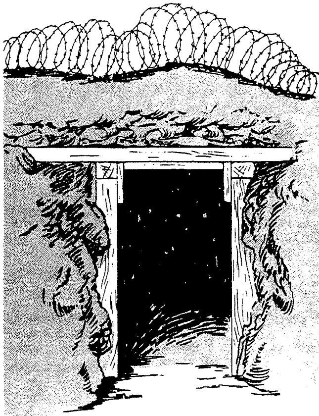
Figure 8-2.—Protective wire on top of overhead cover.
